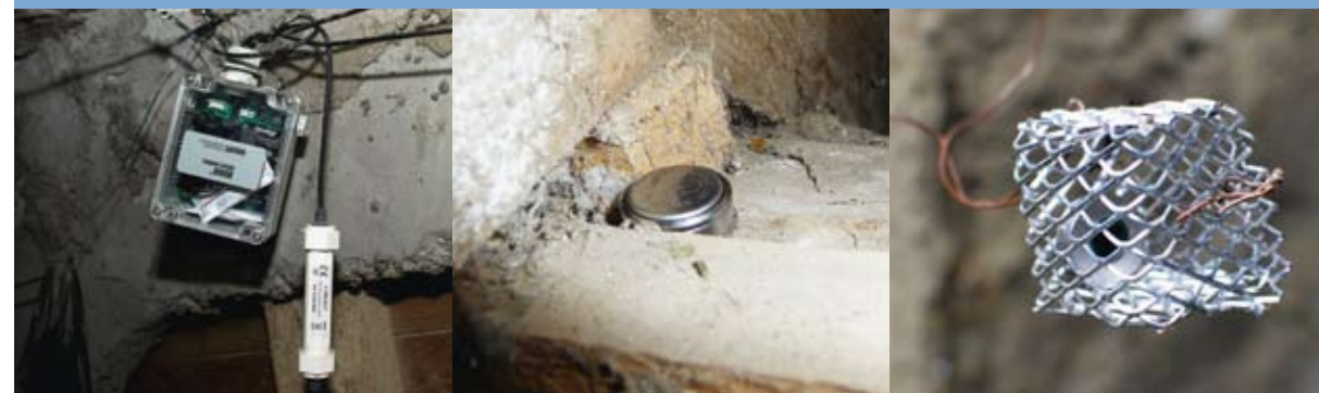
Photo 8 : Data-loggers used to characterize the roosts ( actions A2 and E4 ). Micro-Station HOBO with 4 sensors (to the left), a Thermo-button in place (in the middle), and a Thermo-button in a protective cage hung from a support to limit loss and theft (right).
